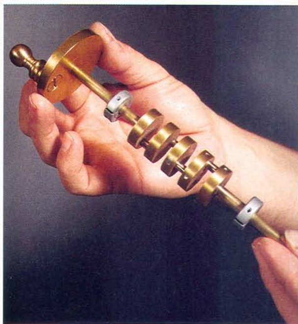
A five-disc crankshaft controller allows the automaton to move in either forward or reverse and at varying speed.
