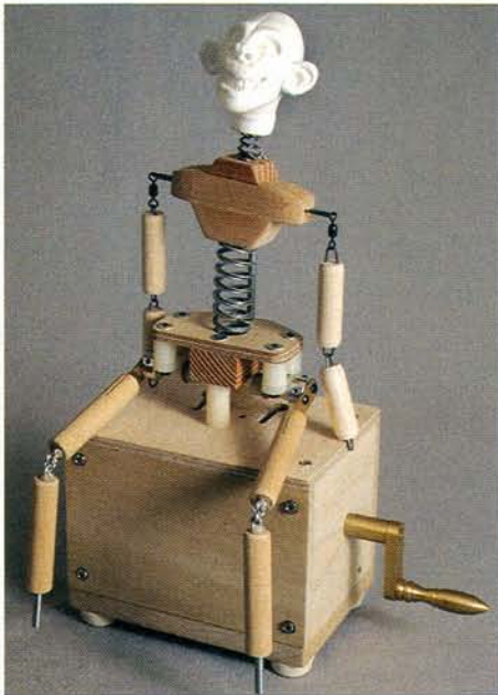
Exposed front view of the automaton armature. The large spring acts as the spine, supporting the upper body.
